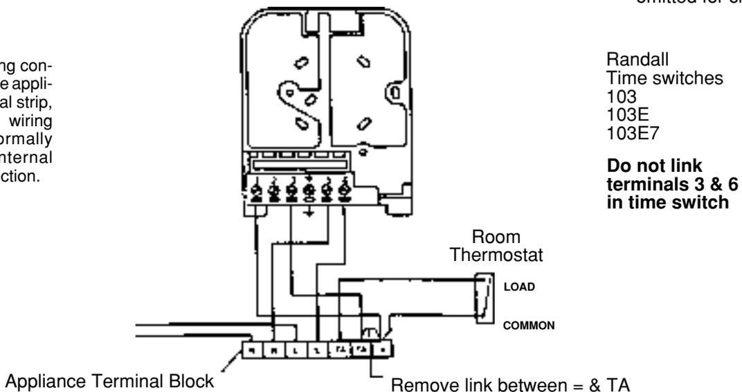
**C. Wiring for 'S' Plan Installations.**
