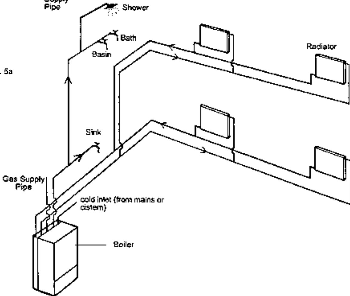
**N.B.** Vokèra Ltd recommend a 2-pipe system. Single pipe systems are more liable to be troublesome unless carefully designed and installed.
