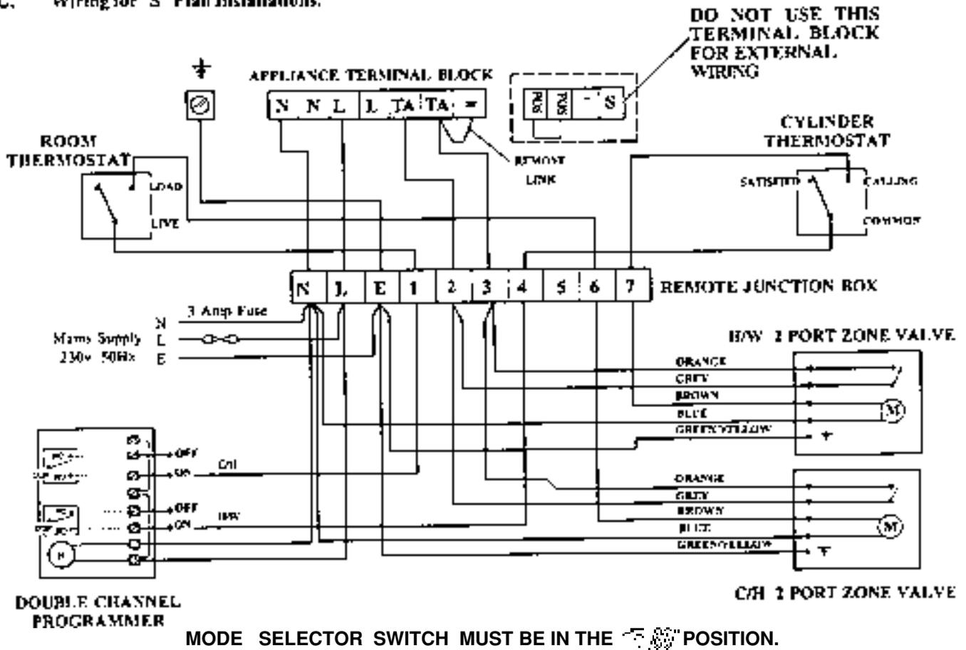
To ease wiring congestion at the appliance terminal strip, remove the wiring harness normally used for internal clock connection.
