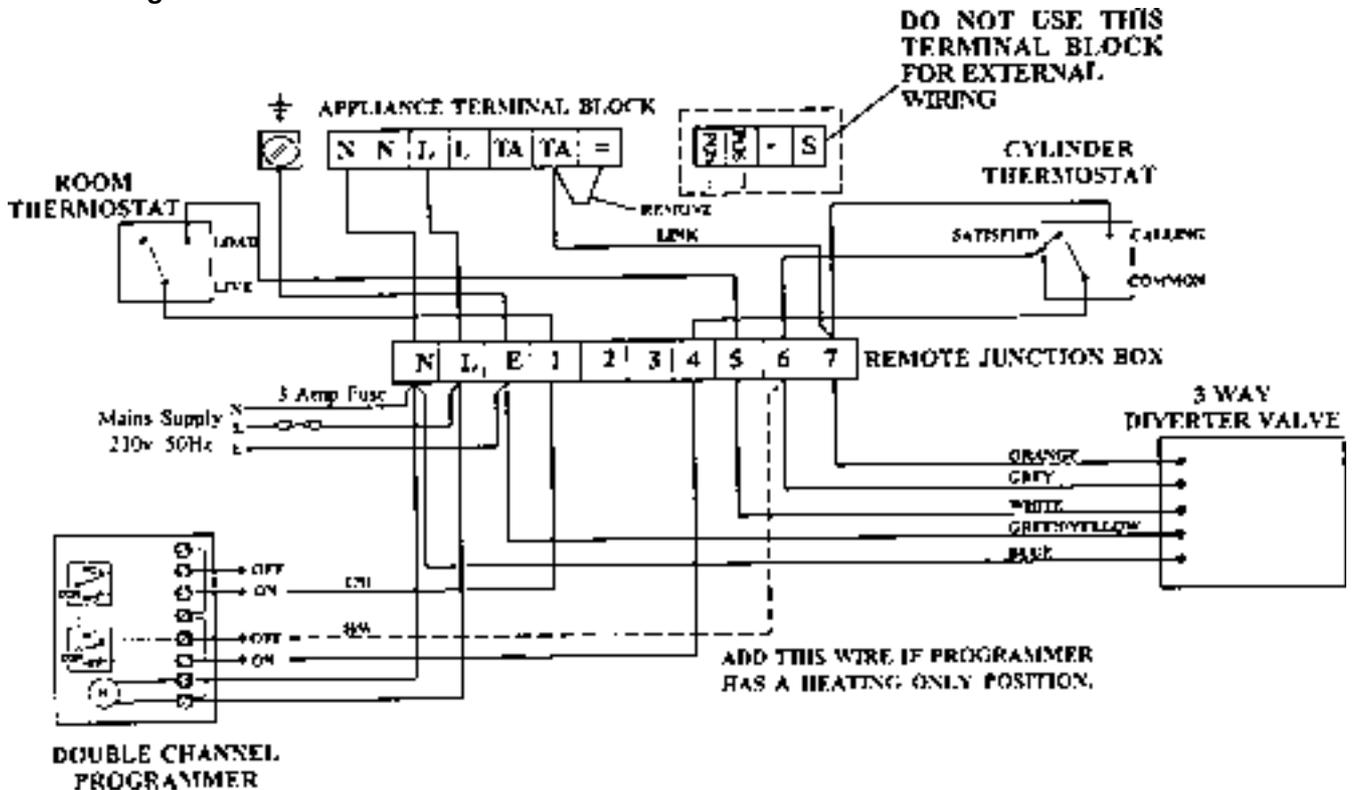
**NOTE: WHEN USING A 'Y' PLAN INSTALLATION THE MODE SELECTOR SWITCH WILL BE OVERRIDEN BY THE CONTROL CIRCUIT.**
