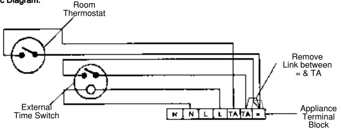
**(ii) ACL Time Switch and Typical Room Thermostat**
